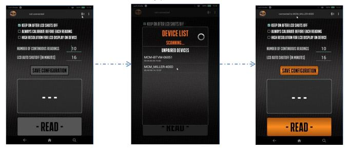
3. Once your 400D device is shown in the **UNPAIRED DEVICES** section, select your 400D... The **pairing process** will complete showing a **connected to...** in the header of the 400D app...
